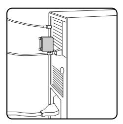
Figure 2-1 Software key installed
