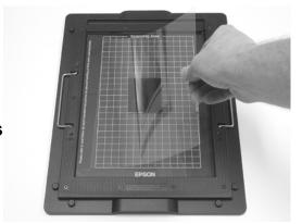
5. Air Bubbles should not be present in the image area. If air is present take a Scanner Wipe and wipe the AZ-42 to remove bubbles.
