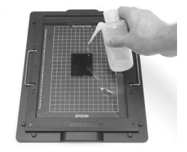
4. Take a pre-cut sheet of AZ-42 Optical Mylar and roll from left to right over the Mounting Bed.
